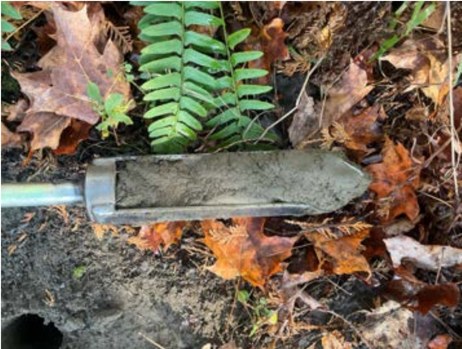
Photo 10. View of soil core sample depicting alluvial deposits.
