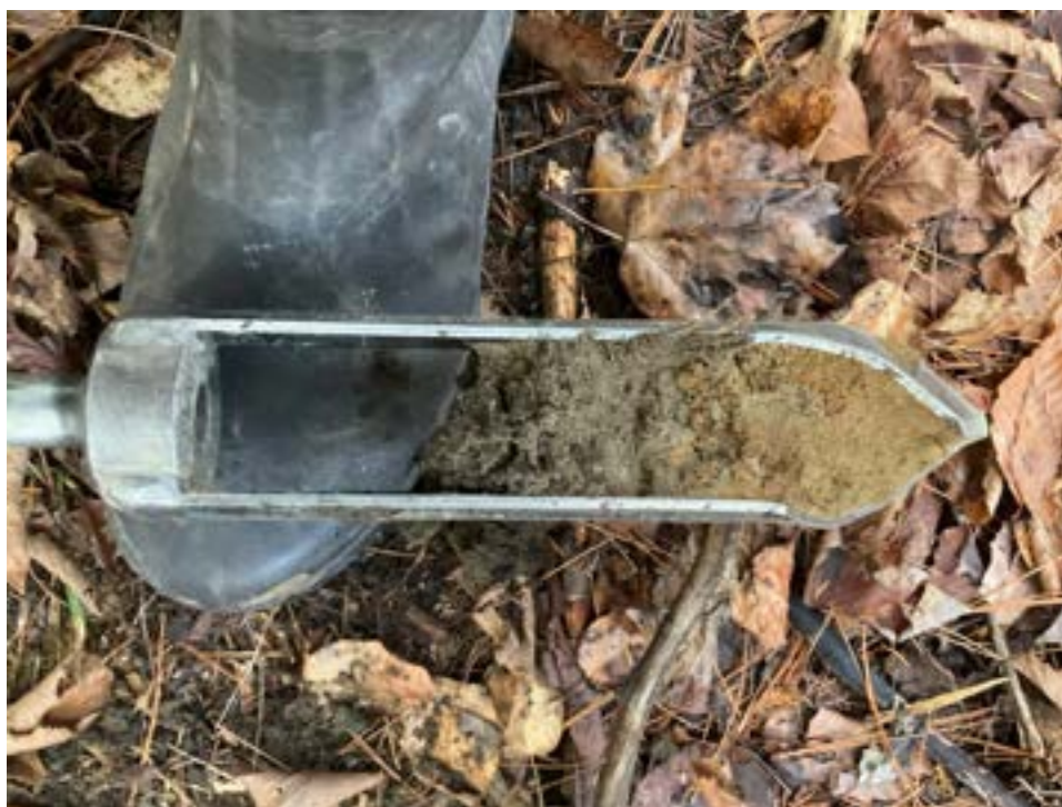
Photo 21. View of soil core sample depicting topsoil and developing B horizon.
