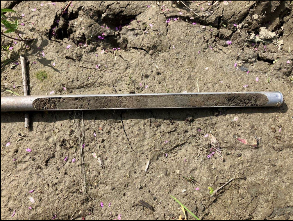
Plate 5. Auger Sample #1 from Proposed Low Floodplain Area Showing Recent Alluvium
