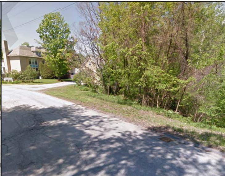
Photo 2. View of the proposed rain garden location showing the catch basin to be capped
